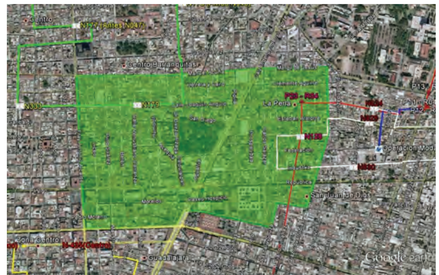
Existing telecoms fibre network, source: Ayuntamiento de Guadalajara
