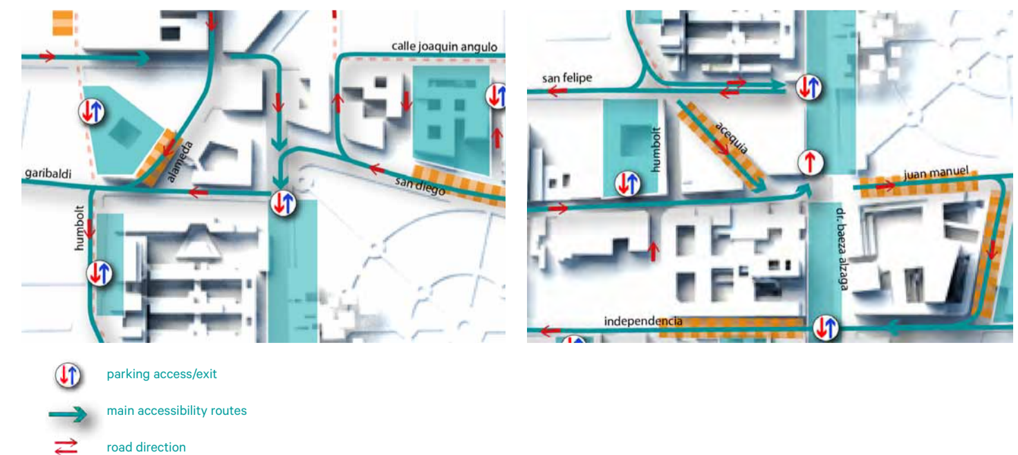
North and south side of the Rambla car park: relation between access ramps and drop-off areas
